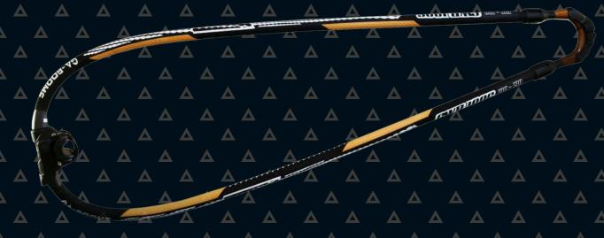
Our newly developed Wave Boom comes in 2 sizes: 140 and 150. A super reduced diameter and partially V shaped grip section give the best ergonomics while the oversized front section gives maximum stiffness. The monocoque molded tail features an intelligent plastic add on component with a rapid outhaul fix system along with a double protection pad for the carbon tail for rock and hard surface encounters.
